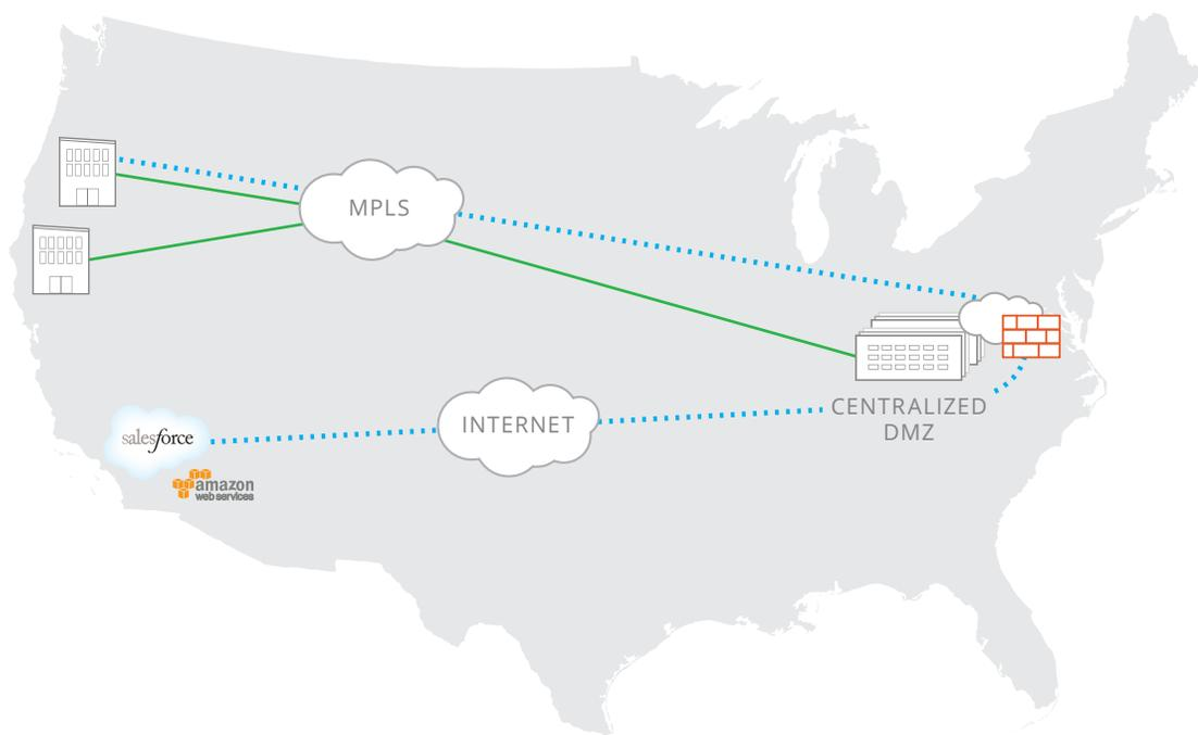
Figure 1: Traffic trombone effect due to centralized DMZ
